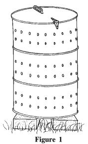
rows of 1/2 inch holes over the length of the barrel to allow for air circulation and drainage of excess moisture. Place the barrel upright on blocks to allow bottom air circulation. Fill the barrel 3/4 full with organic waste material and add about 1/4 cup of high (approximately 30%N) nitrogen containing fertilizer. Apply water until compost is moist but not soggy.
